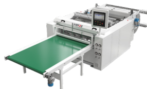
Flying Knife Bottom Seal Bag Machine
